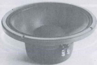
The 2202 is a highly efficient, low frequency loudspeaker. Compared to other loudspeakers having similar sensitivity, its frequency response is unusually linear, varying only 2.5 dB from 100 Hz to 3 kHz. The 2202's performance characteristics make it well suited for use in a small stage monitor loudspeaker, as a midrange driver in wider range sound reinforcement systems or as a low frequency driver in installations where mounting space is restricted.
